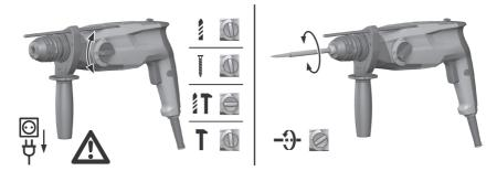
• Set the function selector switch to the "Drilling without hammering action" position  $\frac{1}{2}$ .
