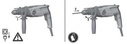
▶ Fit the drill bit or other accessory in the three-jaw chuck or, respectively, remove it.
