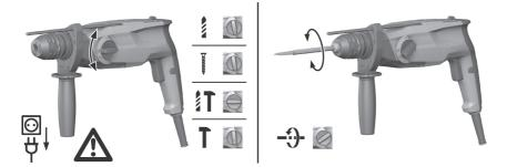
► Set the function selector switch to the "Drilling with hammering action" (hammer drilling) position (1.1)
