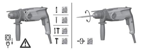
► Set the function selector switch to the "Chisel positioning" position -9-.
