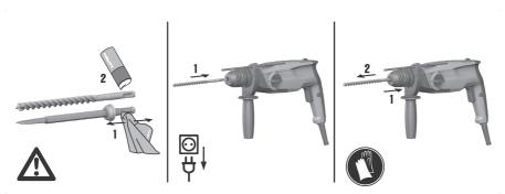
Fit the drill bit or other accessory in the quick-release chuck or, respectively, remove the drill bit or other accessory from the quick-release chuck.
